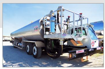
**FLOW METER:** One meter, 600 gpm rated and panel mounted TCS 3000 included as standard equipment (options available).
