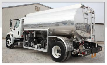
**DEADMAN AND PRESSURE CONTROLS:** Electrically operated in-line deadman/pressure control valve provides primary pressure control. Secondary pressure control regulated by mechanical hose end control valve.
